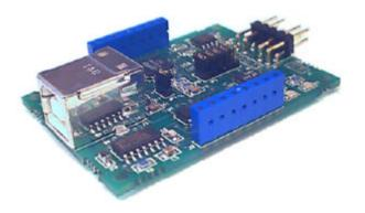
The **USB EasyTap** module is a generic USB <> serial converter and provides a painless way to get your project interfaced to the otherwise complex USB port on your PC. No need to worry about writing your own device drivers since they are included. It can be used in several different ways depending on your needs. By adding a standard TTL <> RS-232 level converter it works like a high speed USB <> RS-232 adapter (with or without hardware handshaking) and you can use it to
