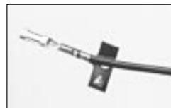
Done. Give the bare-wire ears a final crimp to ensure good contact, and break off the carrier-strip tab.
