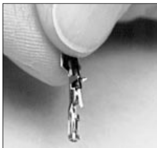
Grasp the wire and socket, using carrier-strip tab as a handle.
