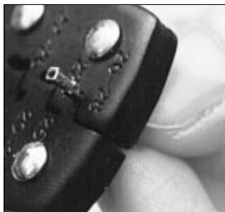
Put the connector into the tool with the ears facing into the die. Squeeze hard.
