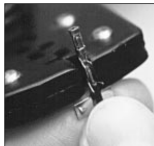
Use the end of the tool and gently pinch the ears to fit the die.
